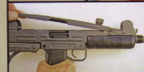
Depress the top cover latch and remove the cover (B).
