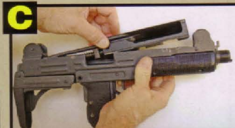
Lift the front of the bolt while moving it slightly rearward, and lift it and the striker assembly out of the frame (C).
