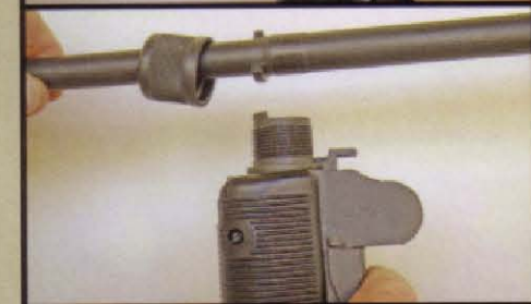
Depress the barrel retaining nut catch, unscrew the nut, and pull the barrel out (A).
