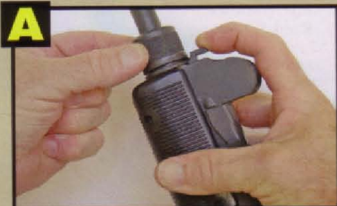
Lift the front of the bolt while moving it slightly rearward, and lift it and the striker assembly out of the frame (C).
