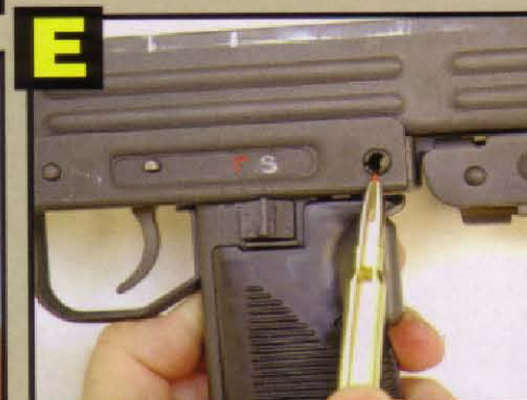
After 5,000 rounds or annually, remove, clean and lubricate the trigger mechanism by pushing this pin through — but not free of — the frame. Then swing the pistol grip down and forward (E). If you need to break your Uzi down further, follow the illustrations in Cornell Publication's reprinted Uzi instruction manual. Reassemble in reverse order.
